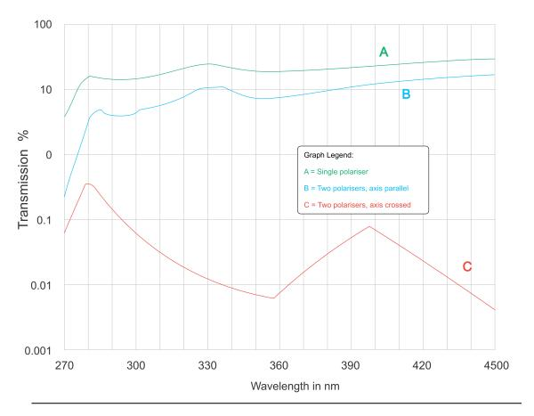
Singe: Transmittance for a single film. Parallel: Transmittance for a double film, axis parallel Crossed: Transmittance for a double film, axis crossed
