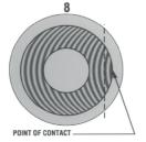
Imaginary tangent line intersects the interference band immediately above it. This shows the sides to be low one band or .0000116" (11.6 millionths of an inch convex).
