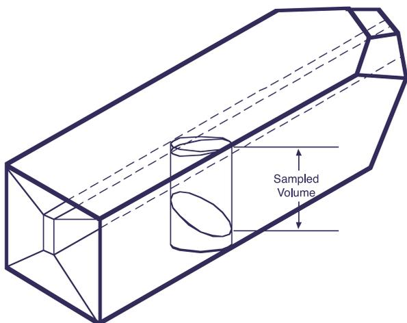
with six 6.35mm diameter circles, each bar is placed on a black background with the minus-X surface facing up. Using side illumination and index matching oil if necessary, each of the marked sites are examined under a stereoscopic microscope
