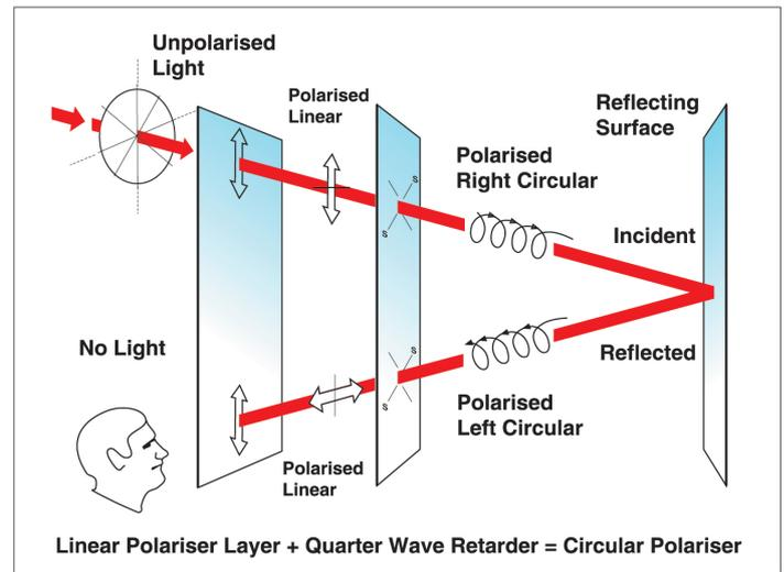
A circular polariser effectively acts like a light valve blocking light completely and therefore offers the ultimate in contrast enhancement.
